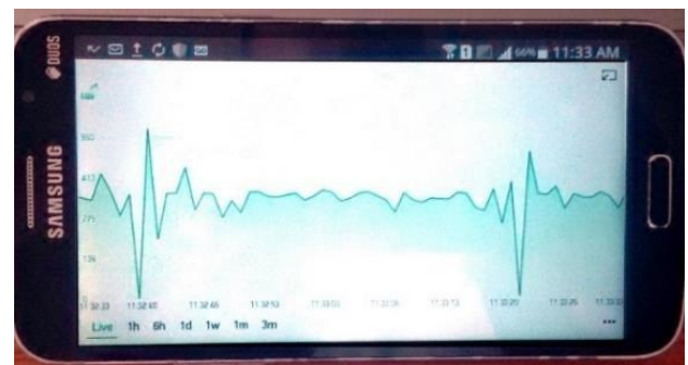
Fig. 8. ECG Output Signal on Blynk Application.
